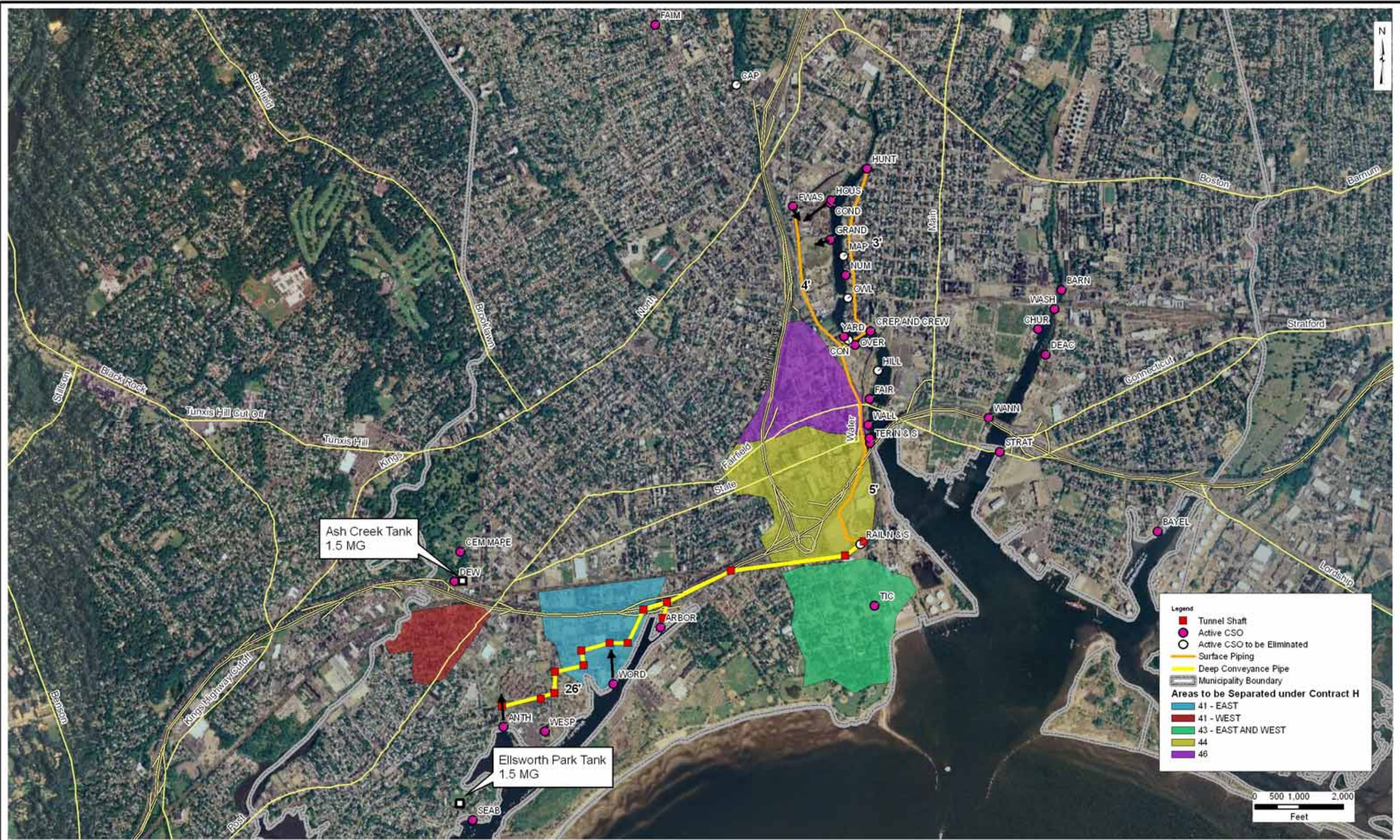
BRIDGEPORT COMBINED SEWER OVERFLOW (CSO) LONG TERM CONTROL PLAN (LTCP) FIGURE 9-1: SELECTED PLAN LAYOUT AND SIZING
