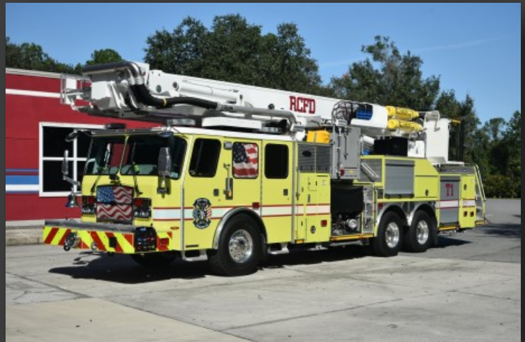
VP Mike Quinn Reedy Creek, FL - Truck 1 - 2018 E -One Cyclone II - 1500/300/117' Bronto SkyLift.
