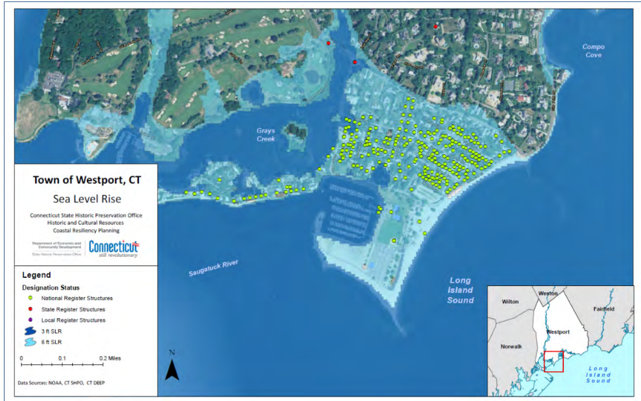
Fig. 13. Predicted extent of flooding in Westport, showing historic properties and town areas likely to be inundated by 3- and 6-foot sea-level rise. Data from NOAA, map by Dewberry and RCG&A.
