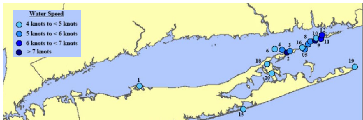
Figure 26-8: Potential Tidal Energy Sites in Long Island Sound. Access available via Long Island Tidal and Wave Energy Study (E3, Inc., 2007).
