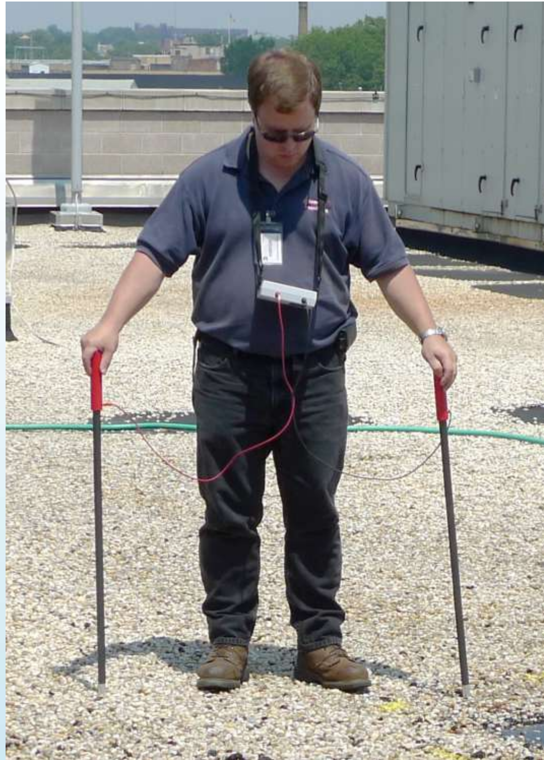
Low voltage vector mapping can be performed on ballasted and gravel surfaced roofs.
