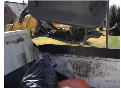
Camera shows driver what goes into hopper
