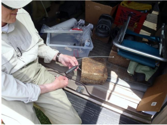
A volunteer prepares a temperature data logger for deployment in a local stream. (Photo courtesy of Candlewood Valley Trout Unlimited)
