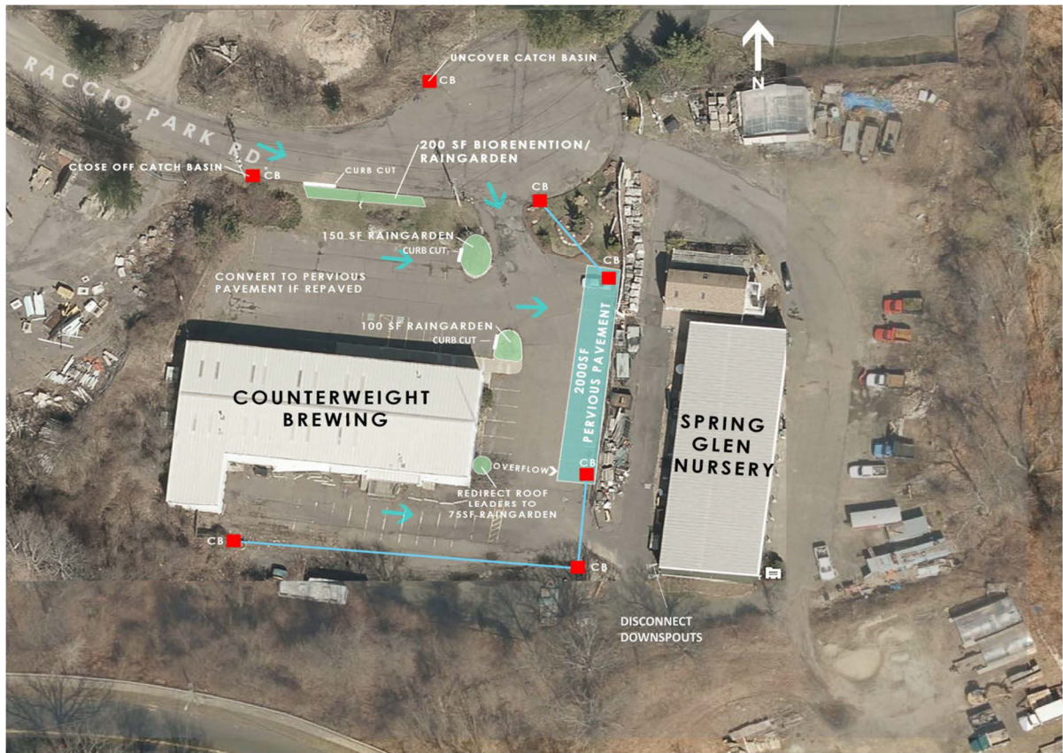
Figure 22. Proposed green infrastructure retrofits for Counter Weight Brewery and Raccio Park Road. "CB" indicates existing catch basin. Blue arrows indicate existing surface flow patterns.
