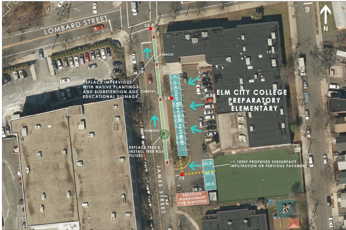
Figure 6. Proposed green infrastructure retrofits for Elm City College Preparatory Elementary School. CB indicates existing catch basin. Blue arrows indicate existing surface flow patterns.
