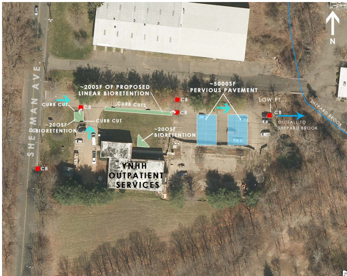
Figure 15. Proposed green infrastructure retrofits for YNHH Outpatient Services Facility. "CB" indicates existing catch basin. Blue arrows indicate existing surface flow patterns.
