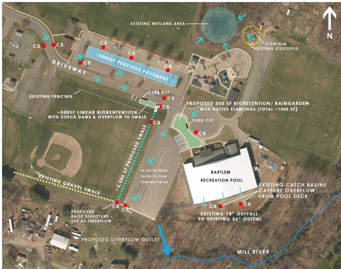
Figure 25. Proposed green infrastructure retrofits for Bartlem Recreation Area. "CB" indicates existing catch basin. Blue arrows indicate existing surface flow patterns.
