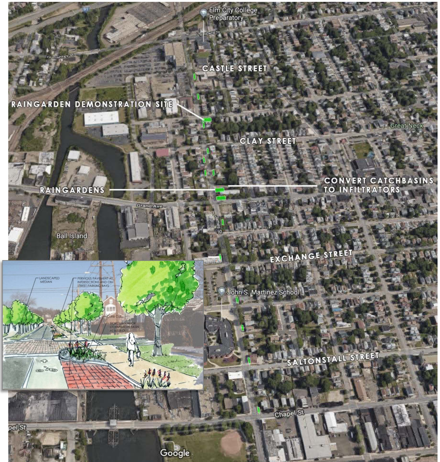
Figure 8. Proposed green infrastructure retrofits for the public right of way, community garden, and condos along James Street. Figure depicts the general concept design of repeating bioswales and/or bump-outs. Locations as marked represent the conceptual pattern, and are matched to suggested locations as much as possible given the scale, but do not necessarily match precisely to specific recommended sites . The inset image demonstrates a street-view rendering of the concept.
