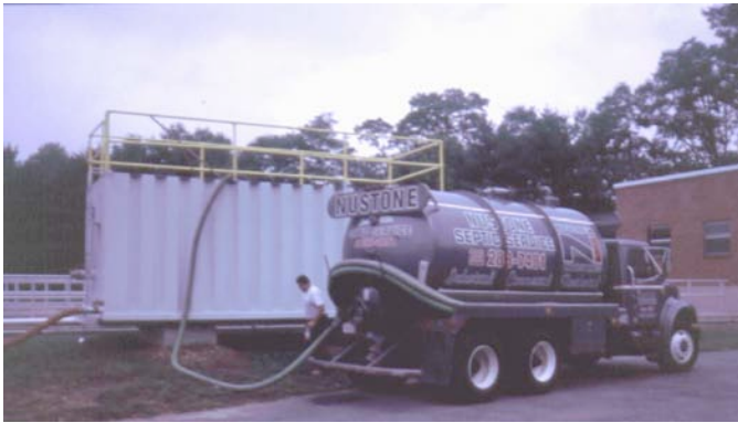
FOG Delivery at Torrington WPCF (Unloading at the Frac Tank)
