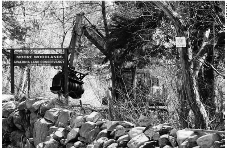
A heavy-duty tree and brush mulcher mounted on a track excavator, called a brontosaurus, mulches a tangle of exotic vines and shrubs at the Avalonia Land Conservancy in Groton. Once the invasive plants are removed, the Conservancy will maintain the area as early successional stage habitat.
