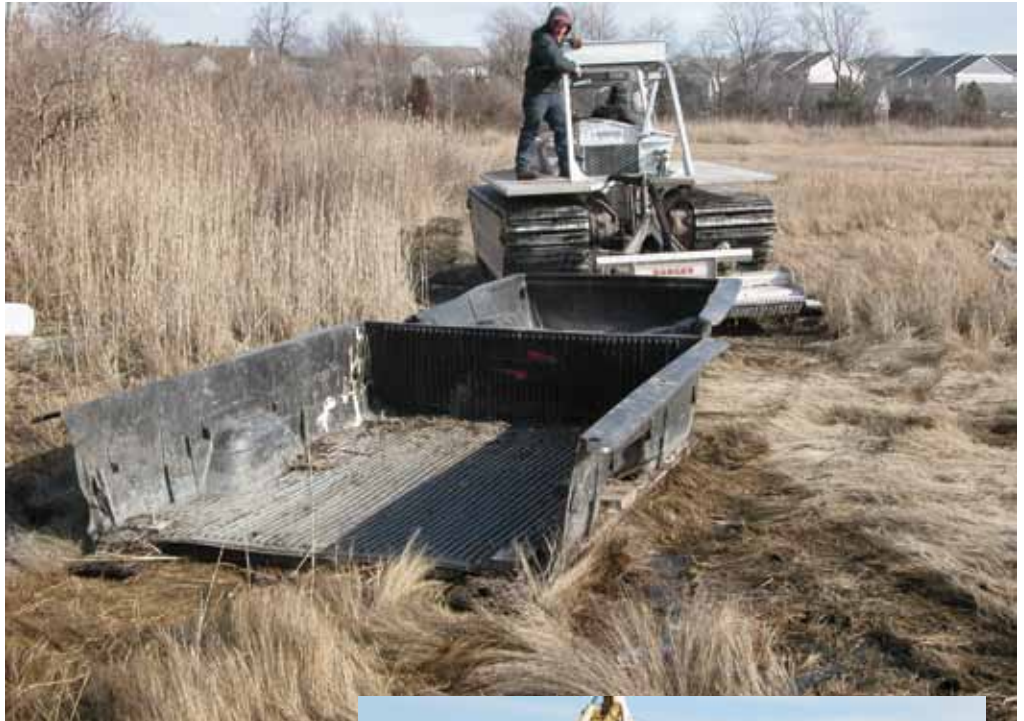
The Marsh Master drags an empty trash sled, designed by the WHAMM crew, to a site for debris removal after Tropical Storm Irene in 2011.
