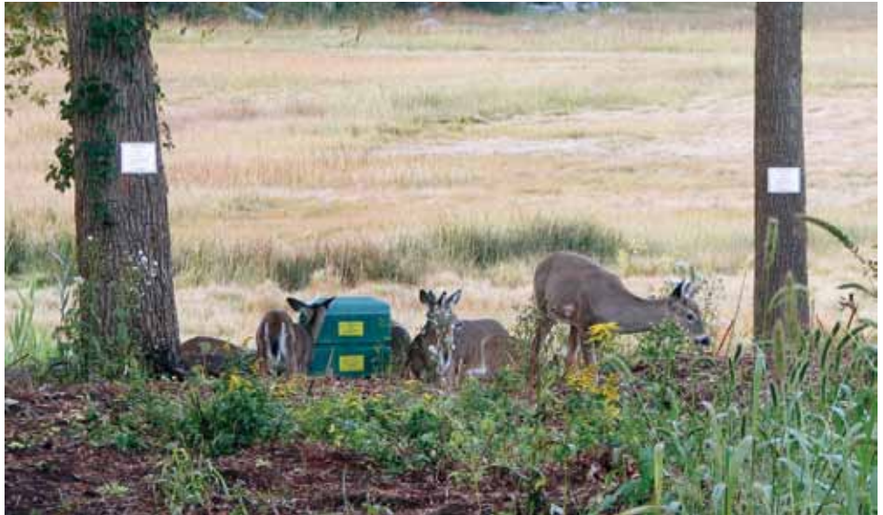
The 4-poster device is a passive feeding station designed to control ticks on white-tailed deer. As deer feed on bait at the station, tickicide-treated rollers brush against the neck, head, and ears where many adult ticks feed.
