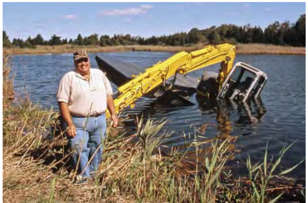
In wetland restoration, things do not always go smoothly, as an experimental pontoon system failed during this vendor field trial.
