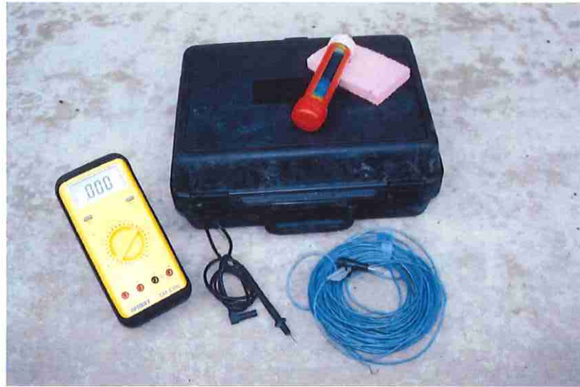
Figure 3. Half-cell corrosion equipment. Clockwise from top: copper- copper sulfate electrode and sponge, lead wires, and voltmeter.
