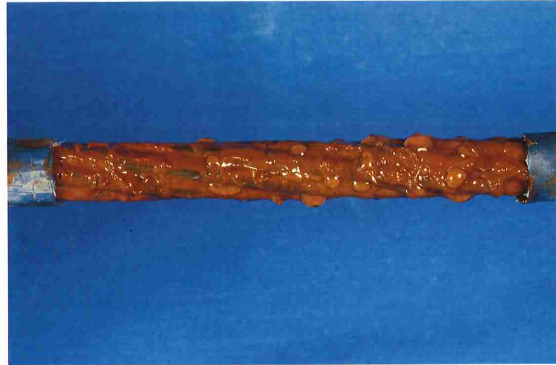
Figure 9. Section of sheathing removed on strand #1 where distilled water has been dripped onto the orange stained grease. L3607 093011 09
