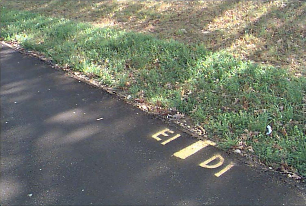
Photo #17. Interface of 1/2 Inch Top Dressing and 1/2 Inch Tilled Compost Sections (October 19, 1998)
