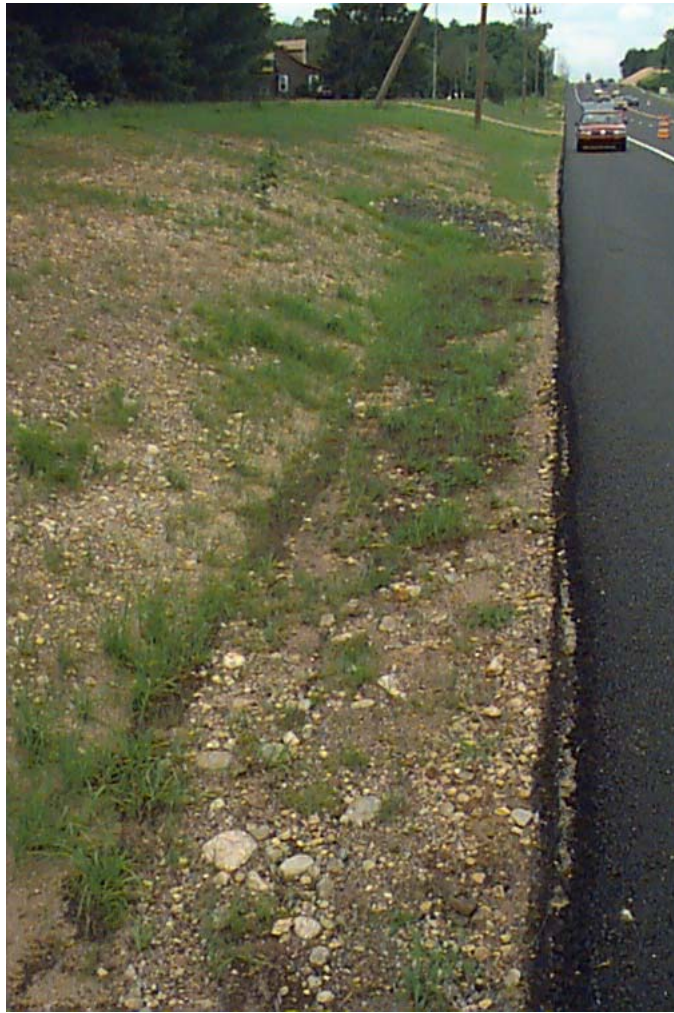
Photo #10. Control Section A1 (June 29, 1998). Dark Areas are Compost that Washed into Section
