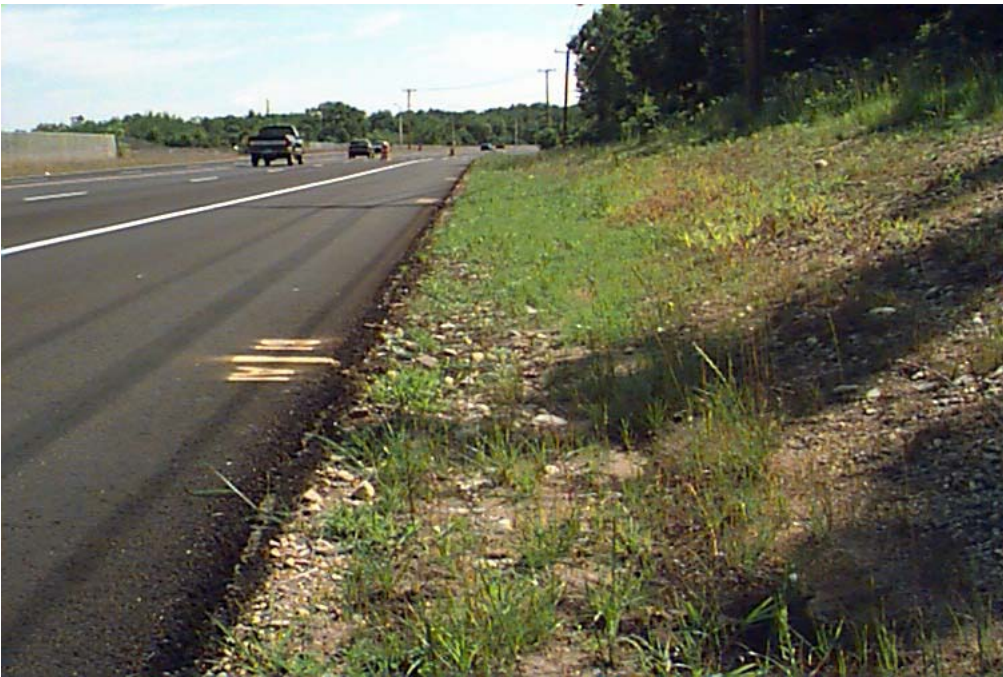
Photo #12. Lower Half of Photo is Control; Upper Half is Section with 2 in. of Compost (July 24, 1998)
