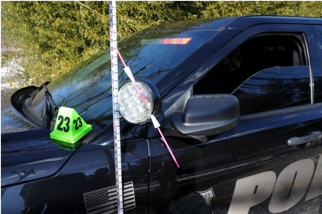
Vehicle #2 (Lieutenant Rosenbaum): Ford Interceptor SUV bearing Connecticut registration 196 SF parked facing a western direction on Main Street Putney. This vehicle had a defect in the driver's side spotlight consistent with being struck by a projectile.
