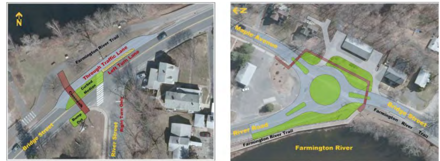
Exhibit 6: Proposed traffic Calming Measures in the study area in the 2014 POCD. Note – the concept plan to the left is mislabeled and should apply to Center Street based on conversations during the RSA.
