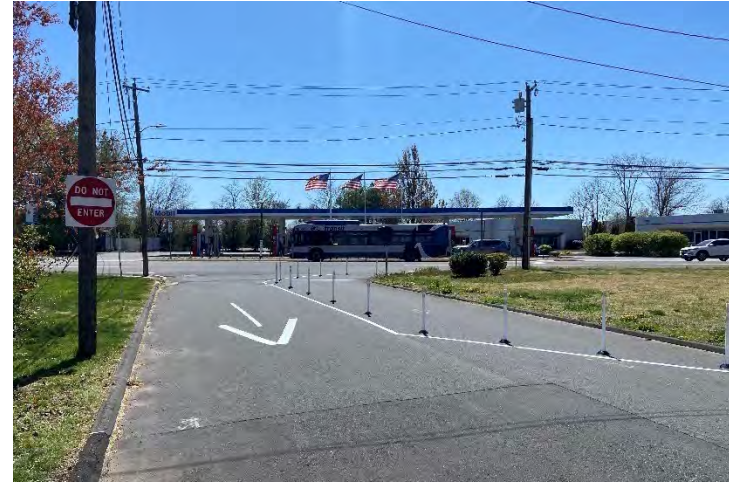
Exhibit 44: A yield-controlled neck down can serve as a gateway to slow traffic entering a neighborhood. This is suggested on Thayer Avenue at Atwater Road to reinforce one-way restriction on Thayer Avenue at Route 565 (Maple Avenue). This can also be tested temporarily with flexible delineators. Source: Federal Highway Administration
