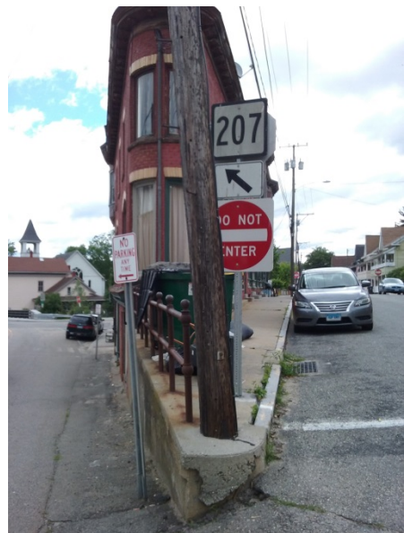
Figure 12. Do Not Enter Sign Blocked by Utility Pole
