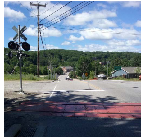
Figure 8. Curvature in Roadway Prevents View of Crosswalk
