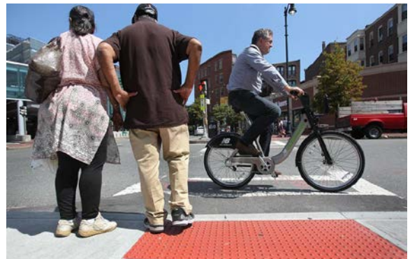
Figure 15. Example of Detectable Warning Strips
