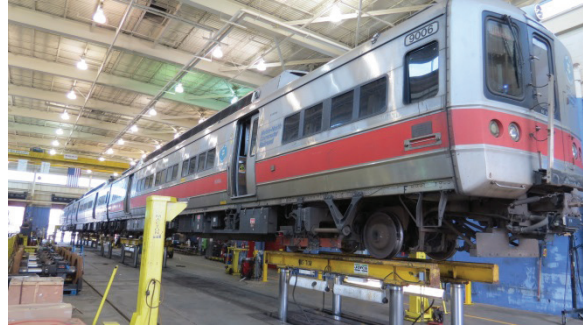
FIGURE 3-23: SEVERAL 35-TON JACKS LIFTING TRAIN
