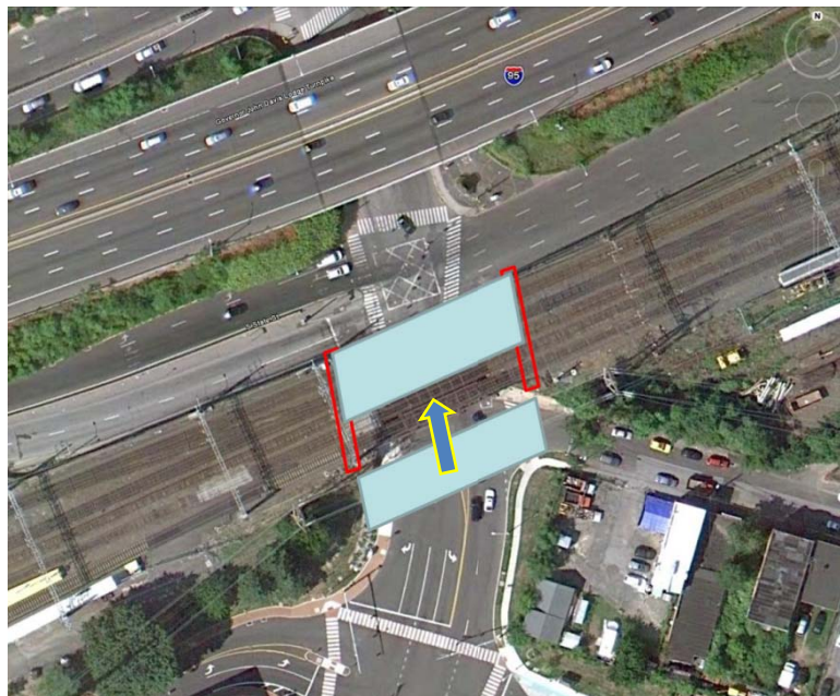
Atlantic Street: Stage 2 Move Northbound Half
