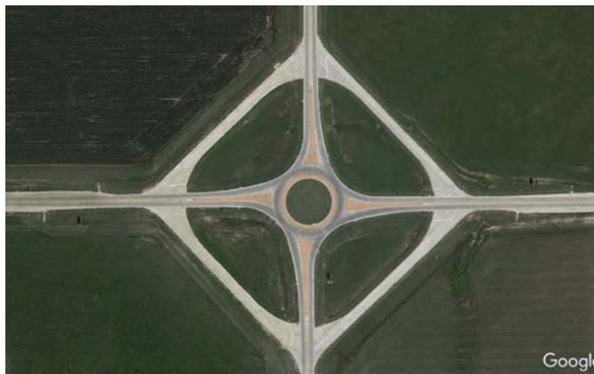
Exhibit 10.40. Example of OSOW bypass lanes.
