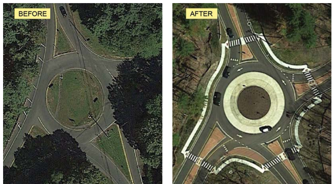
Exhibit 3.10. Example of roundabout retrofit modification.
