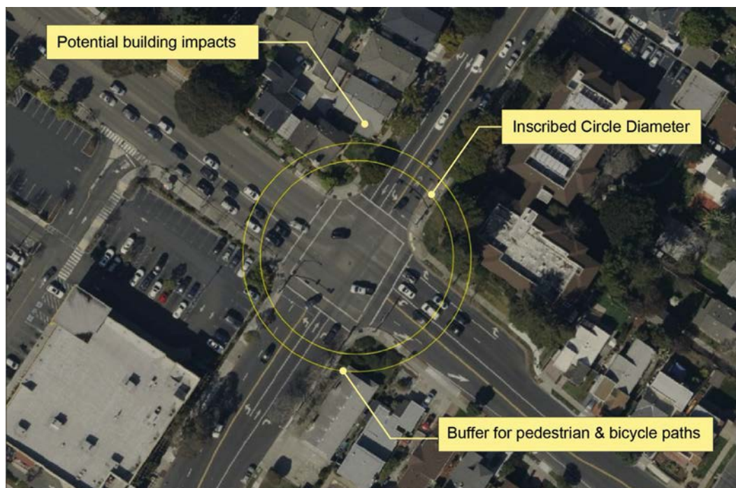
Exhibit 6.1. Example sketch-level roundabout footprint assessment.
