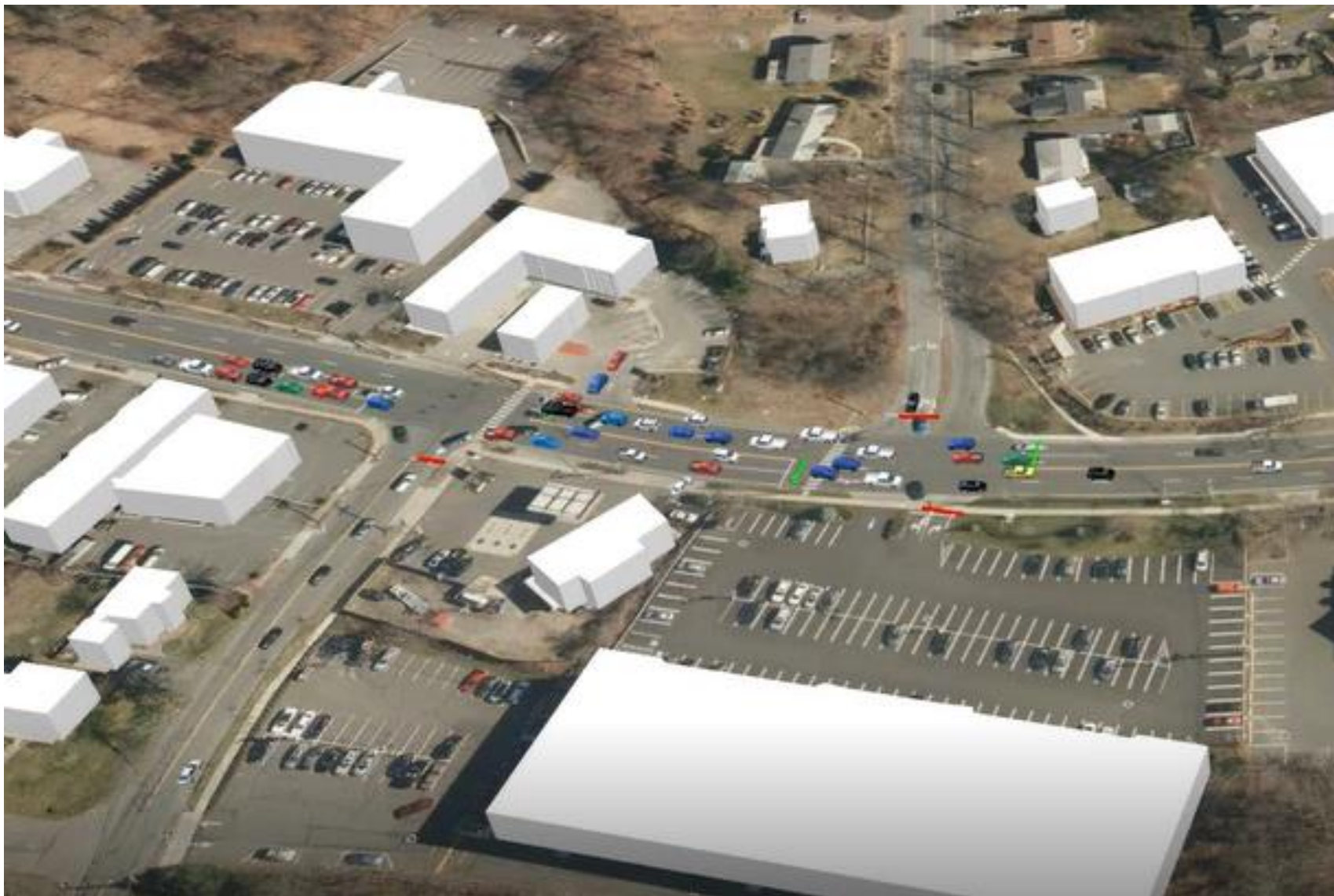
Figure 20: Screen capture of VISSIM traffic model calibrated with PM peak hour drone data
