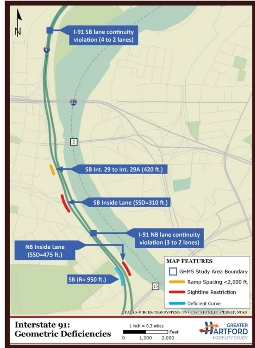
Figure 3-6: Identified I-91 Deficiencies
