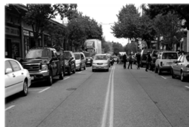
Parking often replaces usable shoulders in village, town center, and urban settings.
