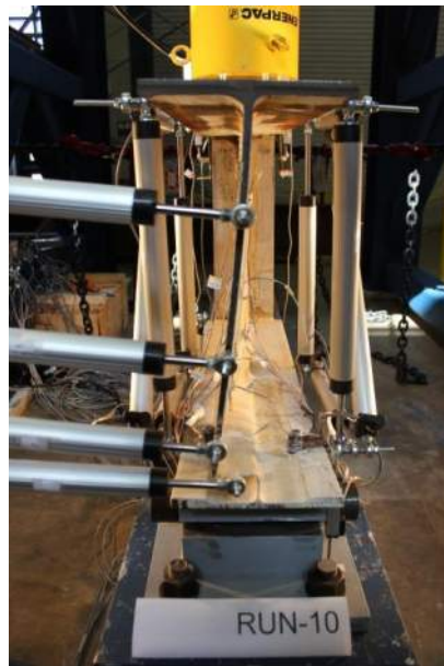
Figure B.2.32 Damaged Girder Longitudinal View: +1.00 in
