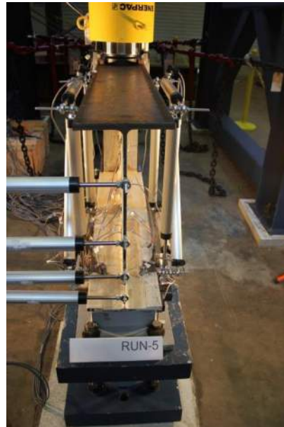
Figure B.2.27 Damaged Girder Longitudinal View: 40 kip
