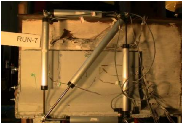
Figure B.3.7 Repaired Girder Right: 84 kip
