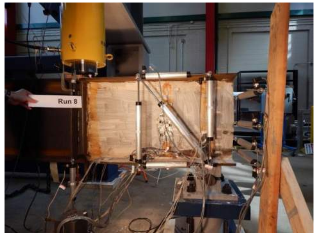
Figure B.1.20 Undamaged Girder Left: Failure
