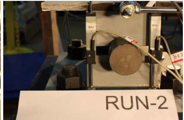
Figure B.2.35 Damaged Girder Bearing: 16 kip
