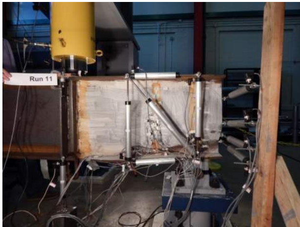
Figure B.1.23 Undamaged Girder Left: +0.75 in
