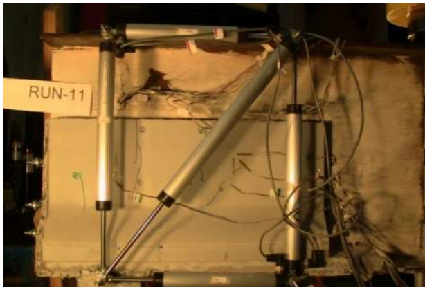
Figure B.3.11 Repaired Girder Right: 140 kip
