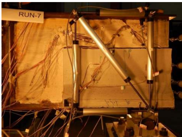
Figure B.3.23 Repaired Girder Left: 84 kip
