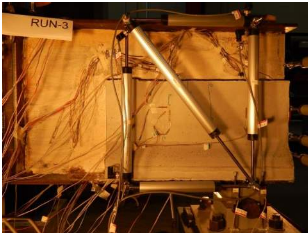
Figure B.3.19 Repaired Girder Left: 36 kip
