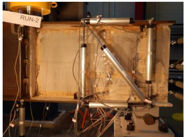
Figure B.2.13 Damaged Girder Left: 16 kip
