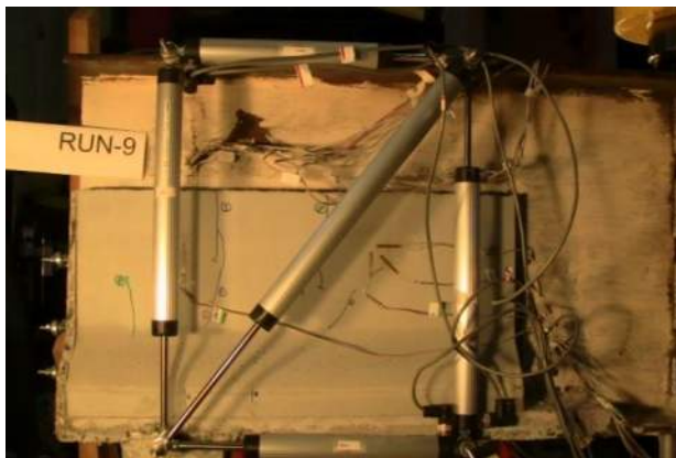
Figure B.3.9 Repaired Girder Right: 108 kip
