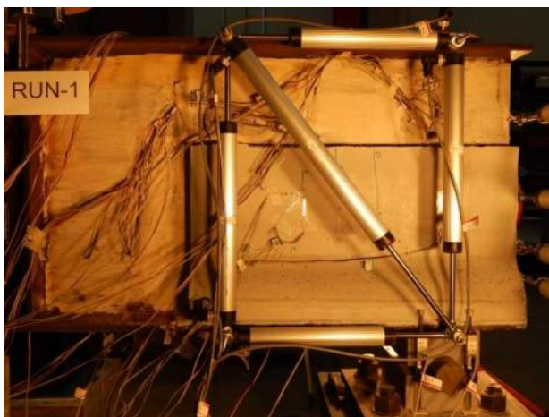
Figure B.3.17 Repaired Girder Left: 12 kip
