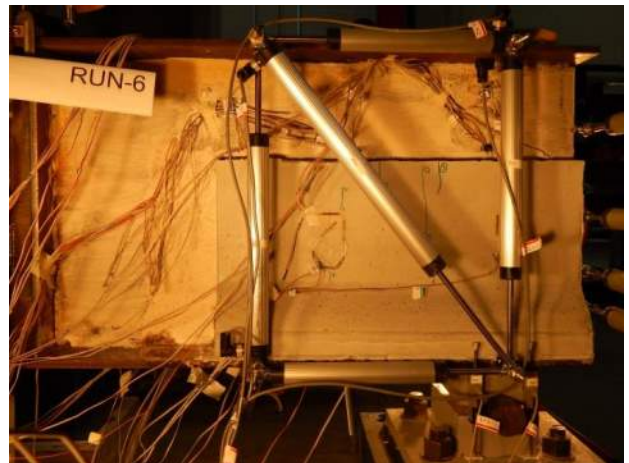
Figure B.3.22 Repaired Girder Left: 72 kip
