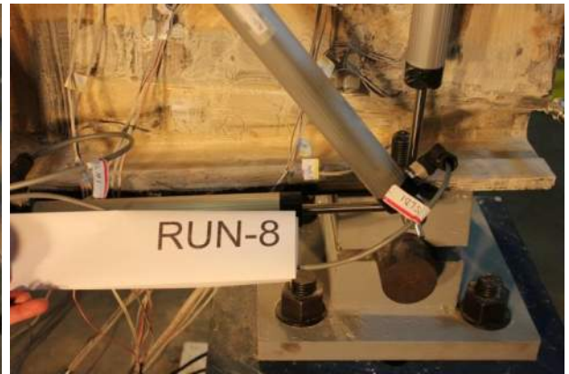
Figure B.2.41 Damaged Girder Bearing: +0.50 in
