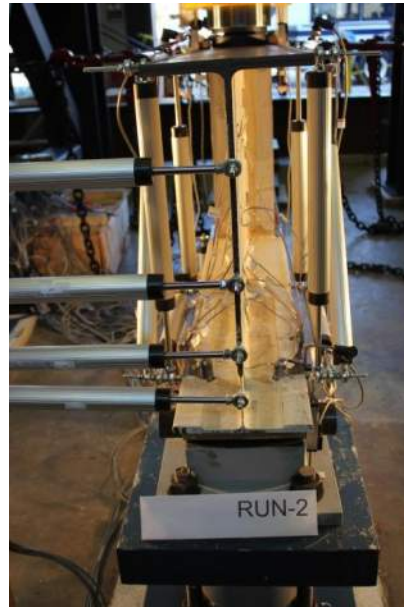
Figure B.2.24 Damaged Girder Longitudinal View: 16 kip
