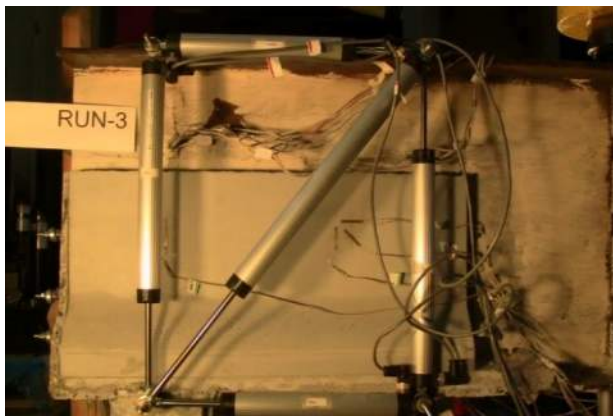
Figure B.3.3 Repaired Girder Right: 36 kip
