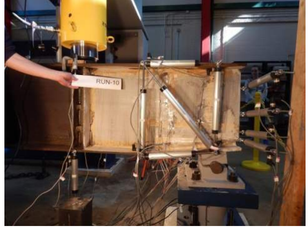
Figure B.2.21 Damaged Girder Left: +1.00 in
