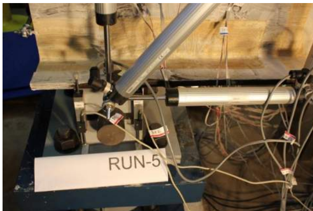
Figure B.2.38 Damaged Girder Bearing: 40 kip
