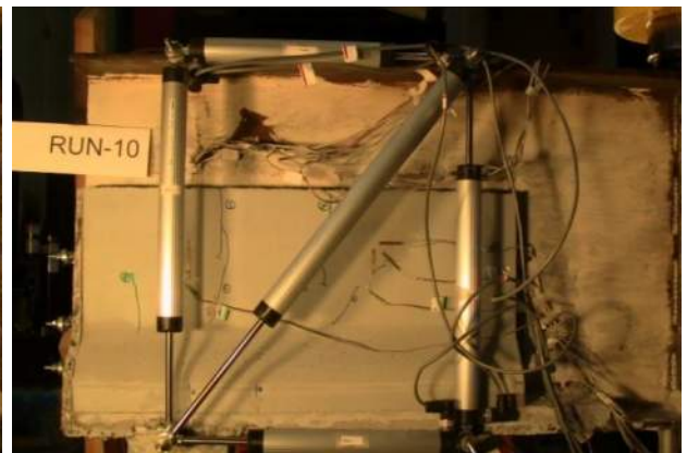
Figure B.3.10 Repaired Girder Right: 120 kip
