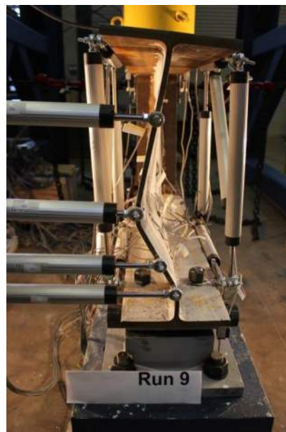
Figure B.1.26 Undamaged Girder Longitudinal: +0.25 in with Load
