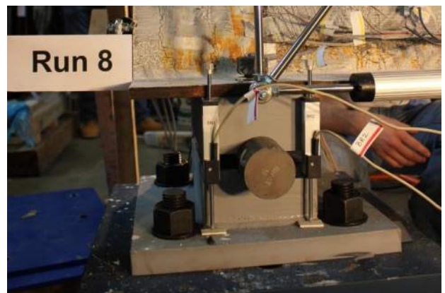
Figure B.1.39 Undamaged Bearing: Failure
