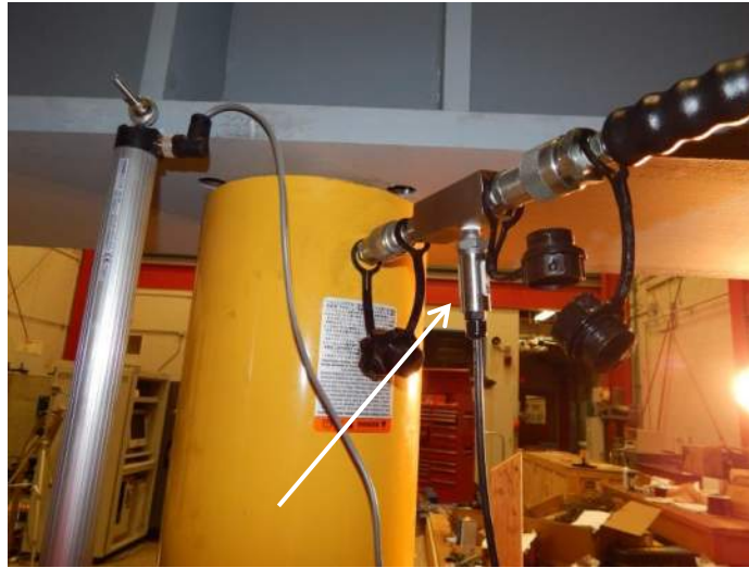
Figure 3.4 Hydraulic Load Ram Pressure Transducer
