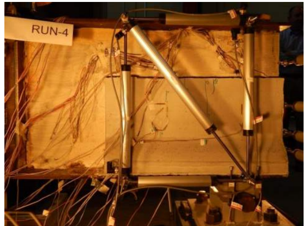
Figure B.3.20 Repaired Girder Left: 48 kip
