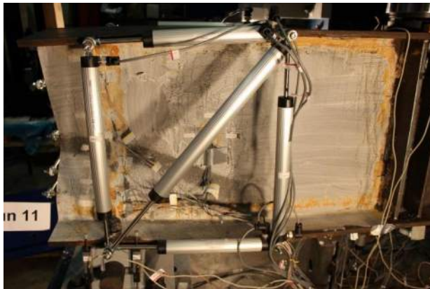
Figure B.1.11 Undamaged Girder Right: +0.75 in
