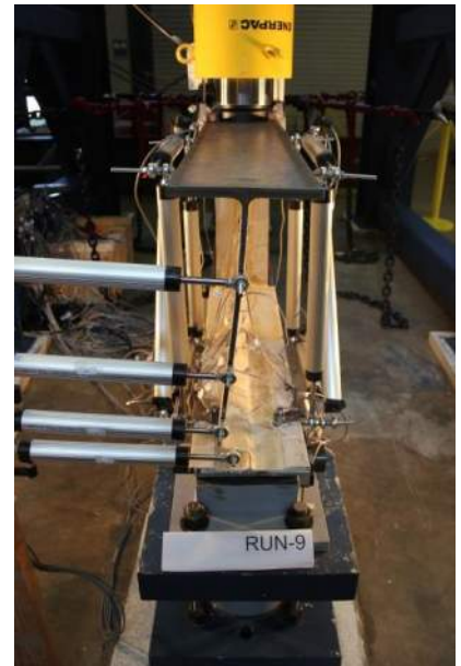
Figure B.2.31 Damaged Girder Longitudinal View: +0.75 in
