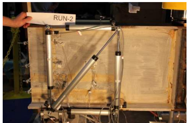
Figure B.2.2 Damaged Girder Right: 16 kip
