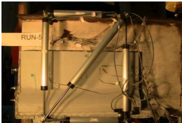
Figure B.3.5 Repaired Girder Right: 60 kip
