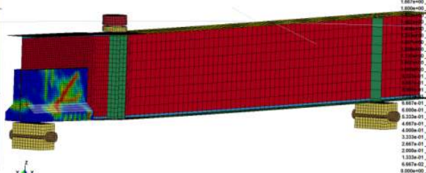
Figure D.3.56 Concrete Scaled Damage: 268 kip
