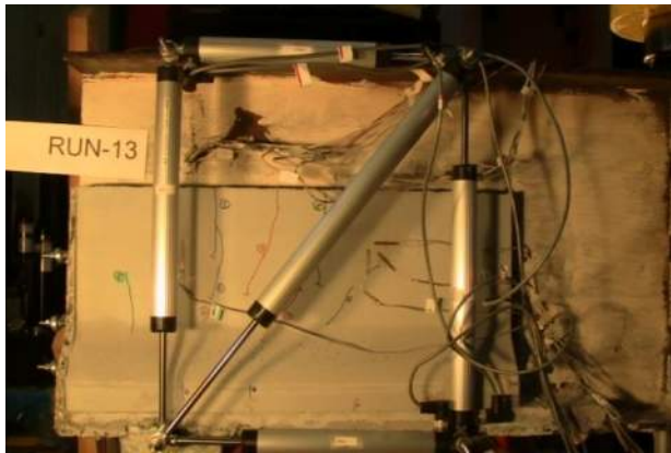
Figure B.3.13 Repaired Girder Right: 180 kip
