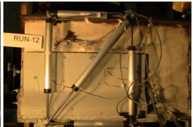
Figure B.3.12 Repaired Girder Right: 160 kip
