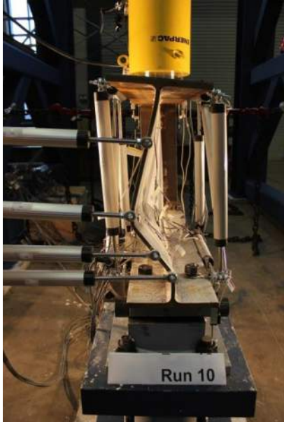
Figure B.1.28 Undamaged Girder Longitudinal: +0.50 in with Load
