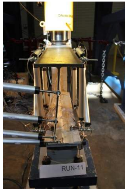
Figure B.2.33 Damaged Girder Longitudinal View: +1.50 in
