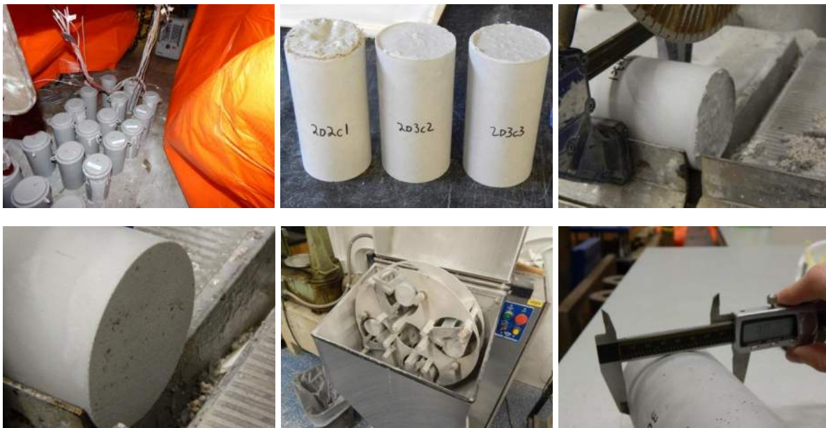
Figure 4.2 Concrete Cylinder Preparation
