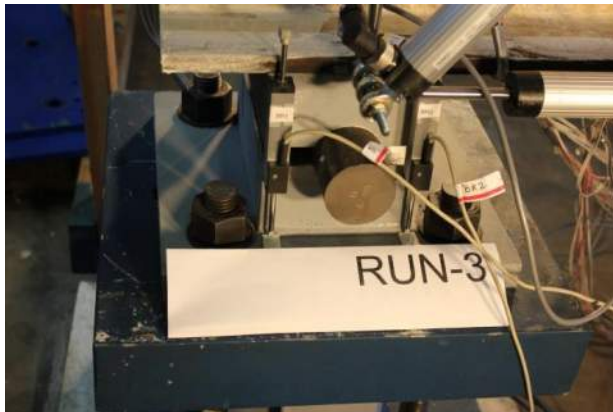
Figure B.2.36 Damaged Girder Bearing: 24 kip
