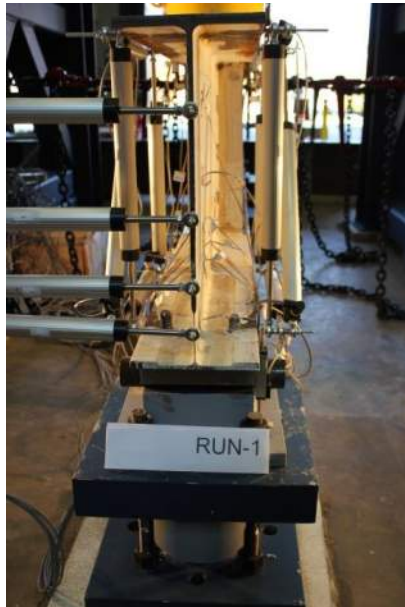
Figure B.2.23 Damaged Girder Longitudinal View: 8 kip
