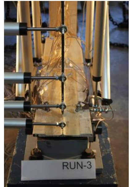
Figure B.2.25 Damaged Girder Longitudinal View: 24 kip
