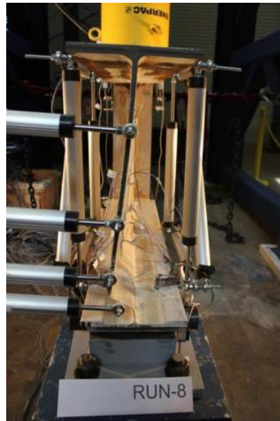
Figure B.2.30 Damaged Girder Longitudinal View: +0.50 in
