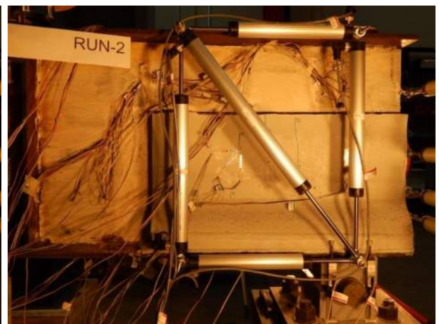
Figure B.3.18 Repaired Girder Left: 24 kip
