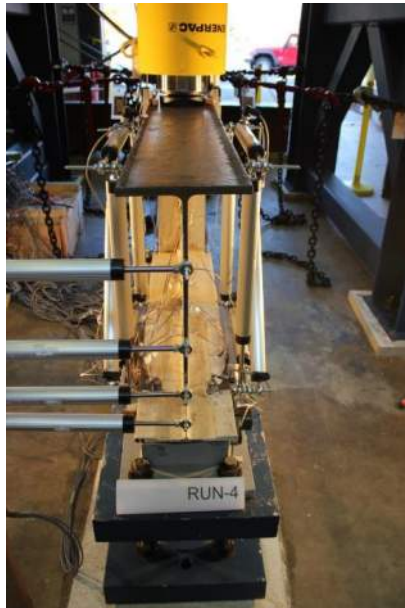
Figure B.2.26 Damaged Girder Longitudinal View: 32 kip
