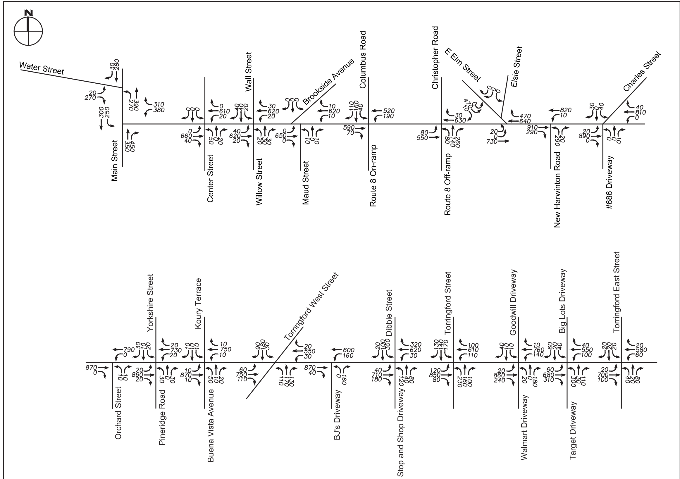
Figure x 2020 Existing Conditions Saturday Midday Peak Hour Traffic Volumes East Main Street Corridor Study Torrington, CT
