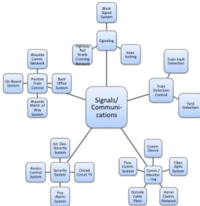
Figure 9. Asset Hierarchy – Fixed Guideway – Rail – Signal/Communications
