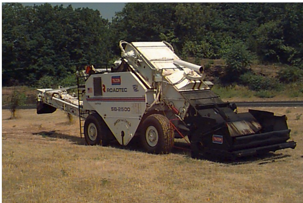
Photo 13. Roadtec Shuttle Buggy Material Transfer Vehicle.
