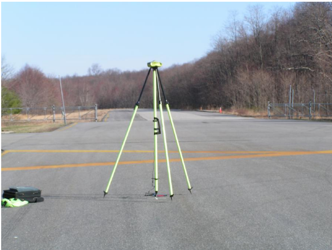
Figure #6 Survey Grade GPS Equipment Used to Locate Points at CU Test Track
