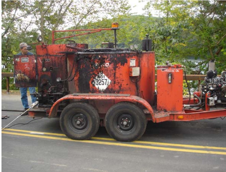
Figure 12 Rubberized Joint Sealant Melting Pot on Trailer
