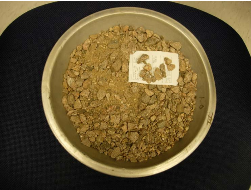
FIGURE 2 Broken stone coarse and natural sand blend fine aggregate used in SuperPave Level 3 mix at Project 28-197 (sample calibrated asphalt content = 5.14%).
