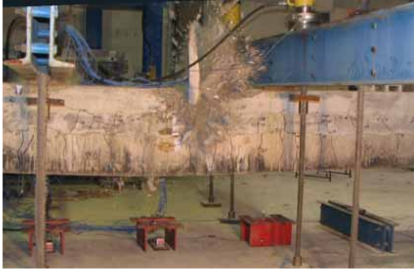
Figure 20. Photo. Failure of Beam 7.
