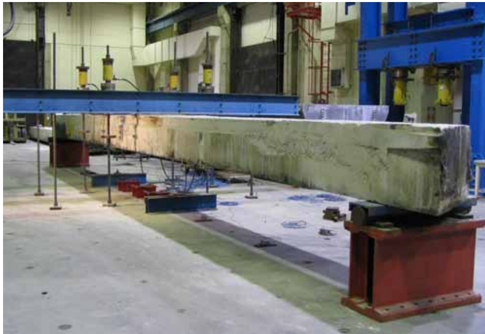
Figure 3. Photo. Flexural loading of a box beam.
