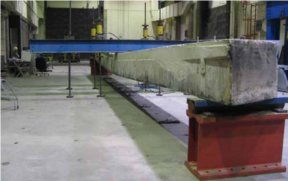
Figure 15. Photo. Deflection of Beam 4 at maximum applied load.
