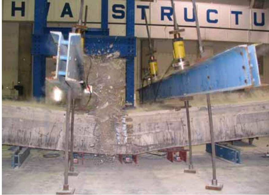
Figure 11. Photo. Failure of Beam 3.
