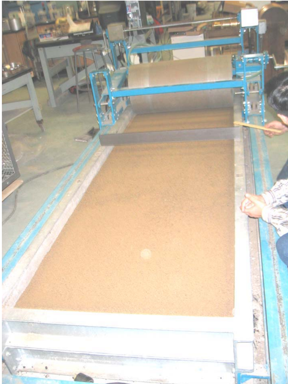
Figure 1. Mold and roller for constructing slabs
