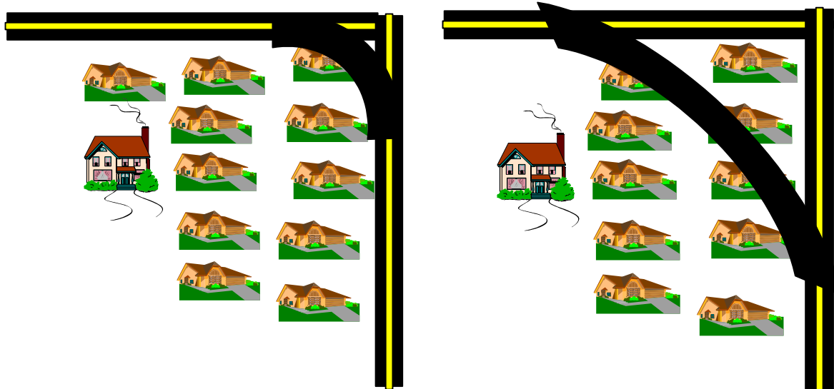
Supplemental Figure: Small Radius of Curvature vs. Large Radius of Curvature
