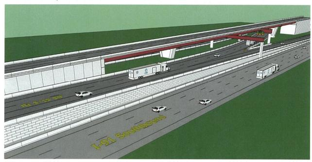
This alternate consists of a 5 span continuous plate girder superstructure with span lengths from south to north of 140', 175', 175', 175', and 140'. The total length is 805'. The superstructure is comprised of Grade 50 weathering steel built up girders composite with an 8.5" cast-in-place reinforced concrete deck.
