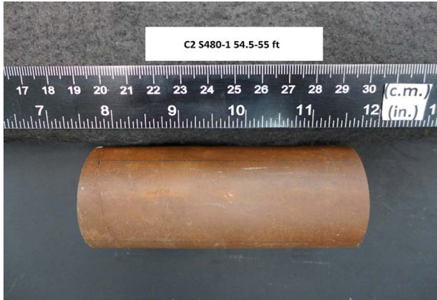
After cutting and grinding
