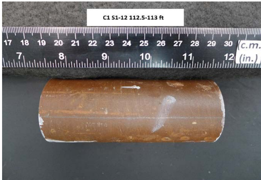
After cutting and grinding
