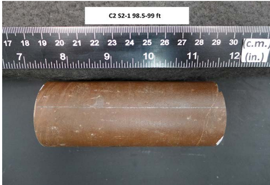
After cutting and grinding
