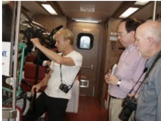
Static Test of M-8 Car Bike Mounts
